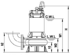
C.W.L : Continuous running water level L.W.L : Lowest running water level
